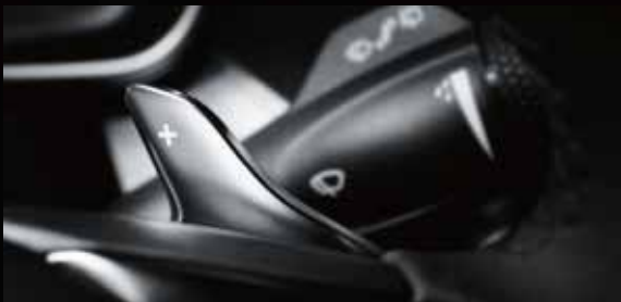
Paddle shift enables complete control over gearbox with hands on the steering wheel
