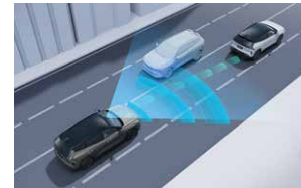
Lane Keep Assistance (LKA) Lane Departure Warning (LDW) Lane Departure Prevention (LDP) LKA=LDW+LDP
